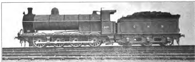
Fig. 5035. Eight-Coupled Goods Locomotive. Great Northern Railway. Cylinders 19 1/4 in. x 26 in.; Working Steam Pressure 175 lbs. per sq. in.; Total Heating Surface 1,138.84 sq. ft.; Diameter of Drivers 56 in.; Weight on Drivers 122,340 lbs.; Total Weight 122,340 lbs.
